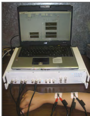
Fig. 2. Measurement set-up for electrode placed on the body
